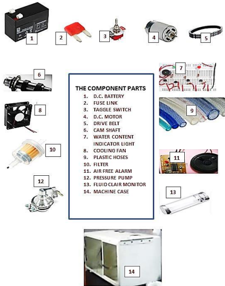
Figure 2. Exploded Components of the Vacuum-type Brake Fluid Bleeder and Recovery Machine
